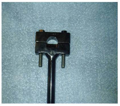
Above is a homemade action wrench used for Mauser and Springfield bolt action receivers. Such a wrench is necessary when replacing or installing a Barrel on a rifle. It's also the action wrench used for the bolt action that is discussed in this book.
