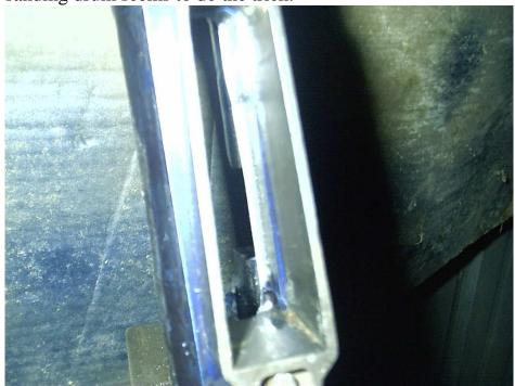
Notice the thin blue line on the rear section of the magazine well opening, it's only a few thousandths thick but is enough to stop the movement of the follower. I found that you don't need to remove a large amount of metal. Grinding the surfaces flush is all that is needed.
