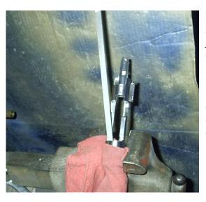
Notice the angle of the file. The Mauser feed ramp is more than just a simple ramp, it's a combination of angles that allows the bolt to rotate, and move forward at the same time. Using a file takes time but you can replicate the ramp. Make certain your files have a safe edge. (Non cutting)
