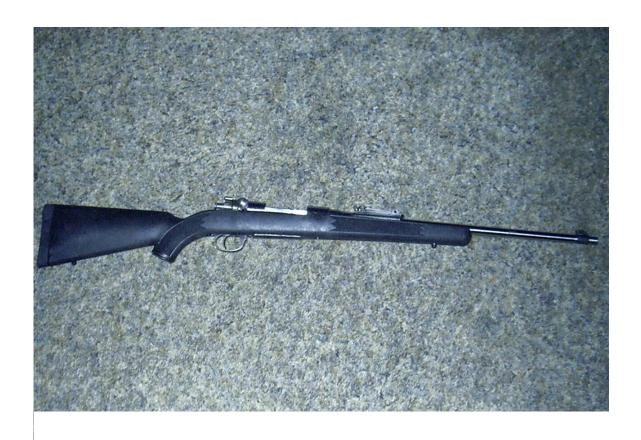
This is the final goal, a shootable Bolt Action Rifle. The stock is an over the counter synthetic stock that is pre-inletted for a large ring Mauser. The barrel is off a 1914 Enfield that was chambered for a 30-06. The barrel has been cut down, rethreaded, and chambered to 308. The barrel was also cut down to accommodate the sights. The sight bases are held in place with a glass bedding compound. The sights are some left over Mauser stuff that I was too lazy to throw away, but hey it works.
