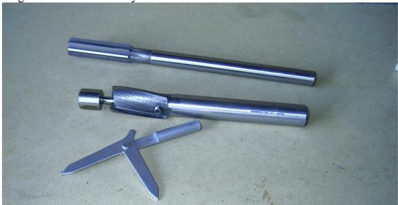
This is the 45/64<sup>th</sup> HSS reamer I use for reaming the receiver blank to accommodate the bolt.
