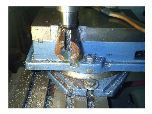
This is the secret to broaching a receiver in the home shop. The gullets of a standard broach will not handle the amount of material needed to cut the raceways of a receiver, but by changing the distance the broach must travel, the impossible, becomes possible.
