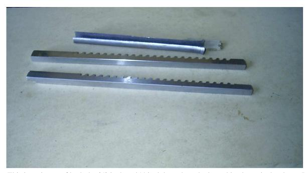
This is a picture of both the 3/8 inch and ¼ inch broaches, the long thin sleeve is the sleeve I made from drill rod for the "C" type broaches to cut the bolt guide slot (1/4 inch broach) and start the raceways.
