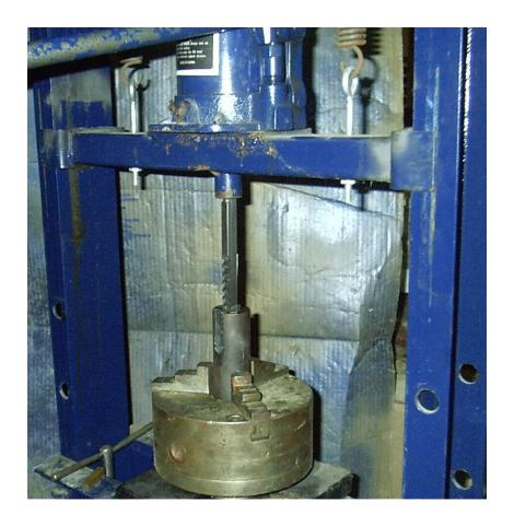
I am now ready to begin broaching the raceway of the receiver. I place the thin sleeve in the receiver blank. I center the slot of the sleeve with the slot in the receiver. It's very important that you get the sleeve centered in the receiver, remember the slot in the sleeve is 3/8 inches wide and the slot in the receiver is 7/16 inches wide.
