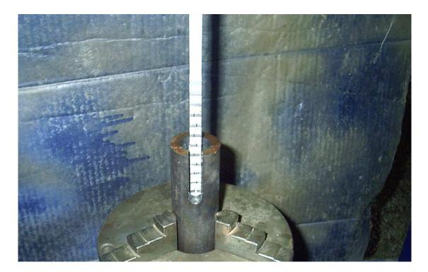
Now reinsert the broach 180 degrees in the receiver blank, align the broach as before and press it down through the receiver blank. The broach should practically fall through the hole leaving two small scratches the full length of the receiver blank. These two lines are still necessary for clearance so don't over look this step.
