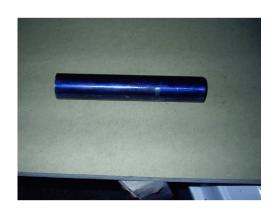
I start the receiver by cutting a piece of 4140 pre-hard 1 ¾ inches in diameter and slightly over 8 ¾ inches long. I center the blank stock in a 4 jaw independent chuck in the lathe for boring. I begin by drilling a pilot hole in the center of the blank stock. I then drill a ½ inch hole at least 4 ½ inches long, using cutting oil. One thing that
