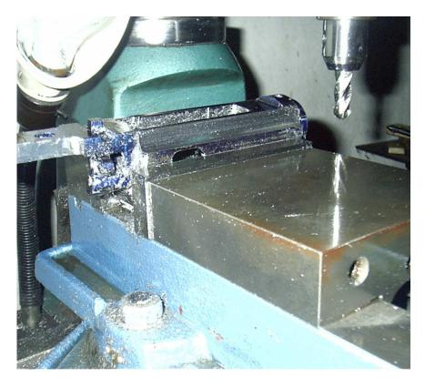
This is how the left lower profile should appear after you have finished the cut. It's very faint in the picture but there is little bright line at the very nose of the front ring, that's the blue layout dye that was removed by the cutter. That how close you need to mill, until you just barely kiss it.
