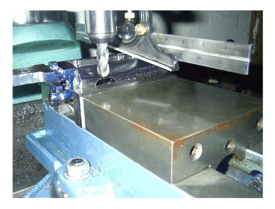
Cut slowly and use plenty of oil. I continue milling until the cut becomes equal the diameter of the front ring. The last few cuts are removing a lot of metal, but don't cut into the front nose of the front ring. Try to make it so your last cut is flush with the nose cut.
