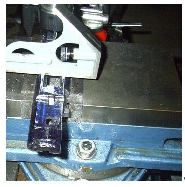
I switch to a 3/16 inch ball end mill, and finish cutting the radius, and the height of the magazine lips. Remember to adjust the vise base to the proper angle.
