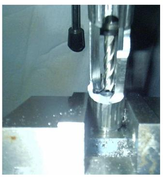
This shows the end mill at full depth in the feed ramp.
