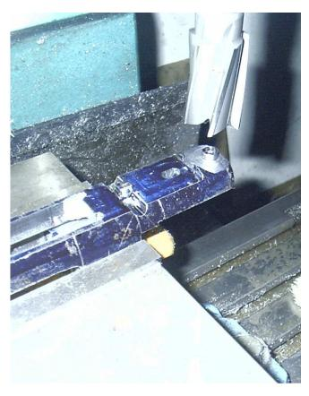
The 1 ¼ inch counter bore is a load for a Mill/Drill, you must go slow and use plenty of cutting oil.
