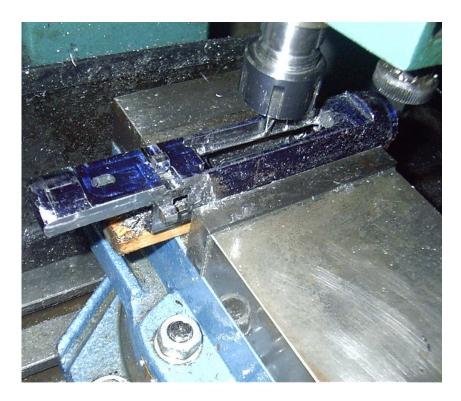
After I have finished putting the final cut on the magazine lips, I take advantage of having the receiver setting flat in the vise and cut the rear hold down lug.
