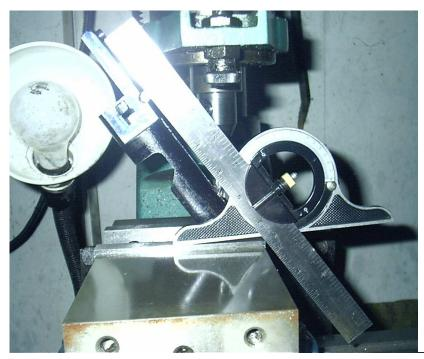
The flat bottom area of the receiver must face toward the spindle and set square to the spindles plane. The combination square base sets flat when setting the receiver to angle. When I was taking the picture it kept falling off the vise that is why the base shows a slight tilt.
