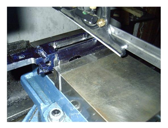
I install a ½ inch cobalt or carbide Ball end mill in the mill, and then lower the end mill to the receiver side, stopping the bottom of the end mill about .050 inches above the thumb slot.
