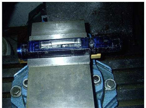
Notice the shape of the magazine that is made by following the scribe lines of template #2. I suggest studying the opening of an actual Mauser receiver before you begin milling
