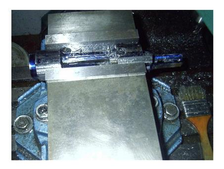
After I finish the top I continue to the right side cutting as before, always making certain not to over cut and using the front nose cut as a guide.
