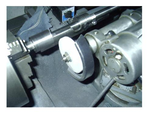
After shaping the profile of the main receiver body the last pass I make with the tool post grinder is the contour at the bottom of the receiver. I have found it matches the diameter of the 3 inch grinding wheel I use to profile the receiver body.
