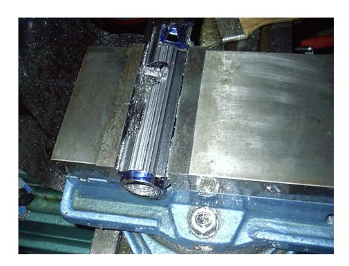
When cutting I raise and lower the cutter and use the table feeds to make the cuts, and do not turn or move the receiver, until I am finished with a side. Now this does leave the surface very rough.
