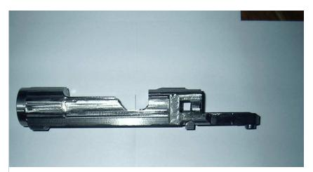
This is the left side of the receiver. The area in front of the bolt stop flange must be shaped smooth for the bolt stop to rest properly against the side of the receiver.
