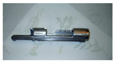
This is the right side of the receiver. The rear of the receiver has been milled down .040 inches more that the front ring. Other than final fitting and shaping, you now have a firearm.
