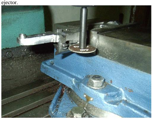
Mounting the bolt stop/ejector box is fairly straight forward. I use a 3mm drill bit to drill the hole. I found out the hard way that you must drill the hole straight.
