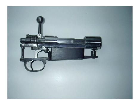
Notice the position of the sear and how it is contacting the receiver toward the rear of the tang.
