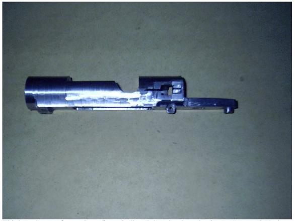
This is a picture of a receiver after grinding. It has the shape but is rough overall. Notice the marks on the lower section of the receiver below the thumb slot, the rubber abrasive wheel all but completely removed those marks.
